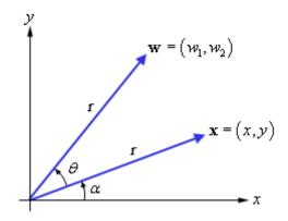
Unlike the previous transformation where we could just write down the equations we'll need to do a little derivation work here. First, from our basic knowledge of trigonometry we know that
