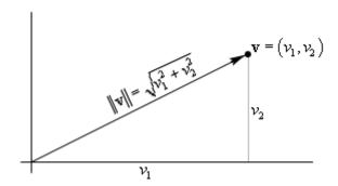
Since we know that the components of  $\mathbf{v}$  are also the coordinates of the terminal point of the vector when its initial point is the origin (as it is here) we know then the lengths of the sides of a right triangle as shown. Then using the Pythagorean Theorem we can find the length of the hypotenuse, but that is also the length of the vector. A similar argument can be done on the 3-space version.
