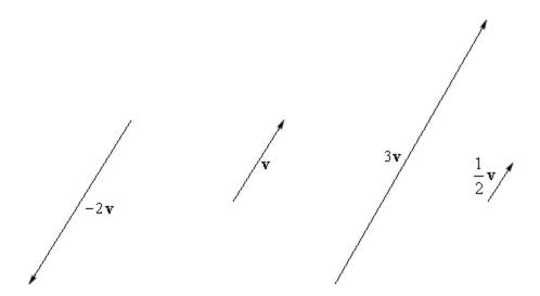
Note that we can see from this that scalar multiples are parallel. In fact it can be shown that if  $\mathbf{v}$  and  $\mathbf{w}$  are two parallel vectors then there is a non-zero scalar c such that  $\mathbf{v} = c\mathbf{w}$ , or in other words the two vectors will be scalar multiples of each other.
