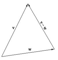
Finally, if we were to go back to the original sketch add in components for the vectors we will see that in 2-space we can compute the difference as follows,
