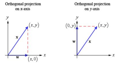
So, we project  $\mathbf{x}$  onto the *x*-axis or *y*-axis depending upon which we're after. Of course we also have a variety of projections in  $\mathbb{R}^3$  as well. We could project onto one of the three axes or we could project onto one of the three coordinate planes.
