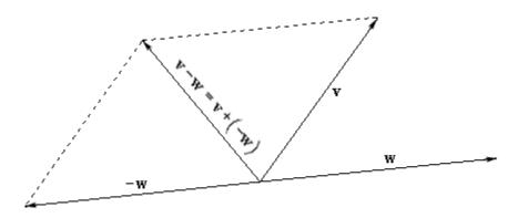
Now, while this sketch shows us what the vector for the difference is as a summation we generally like to have a sketch that relates to the two original vectors and not one of the vectors and the negative of the other. We can do this by recalling that any two vectors are equal if the have the same magnitude and direction. Upon recalling this we can pick up the vector representing the difference and moving it as show below.
